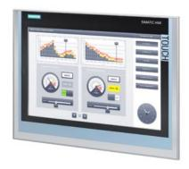
SIMATIC HMI TP1500 Comfort, Comfort Panel, touch operation, 15" widescreen TFT display, 16 million colors, PROFINET interface, MPI/PROFIBUS DP interface, 24 MB configuration memory, WEC 2013, configurable as of WinCC Comfort V14 SP1 with HSP, ambient temperature up to 45  $^{\circ}\text{C}$
