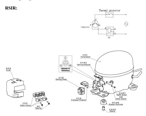
Note: Each of the starting relay, the thermal protector, the terminal cover and the screw assembly is separately provided by our company.
